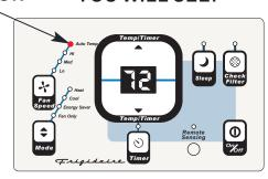
Note: The fan speed will begin in HI, then adjust to MED and LO as the room temperature conditions indictates. For example in cooling, if the room doesn't get too warm it will stay at LO. If the room temperature rises quickly, such as a door being opened, it will automatically go to HI speed. The fan speeds will adjust back to LO as the room returns to the original set temperature.
